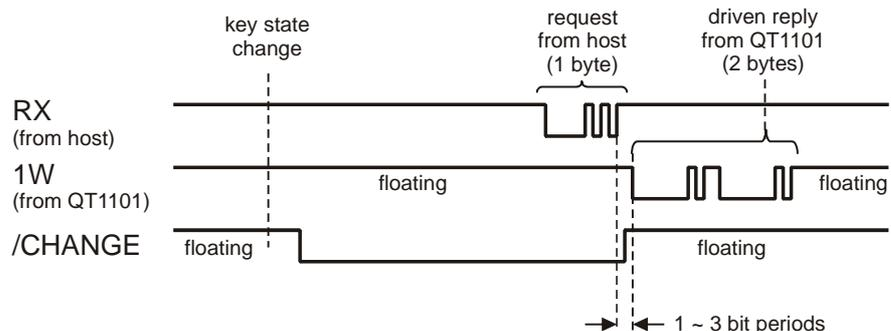
Following a 'P' on Rx, the QT1101 will send the same response pattern (Figure 2-3) over the 1W line as in pure 1W mode.
