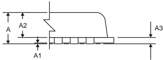
Note that there is no functional requirement for the large pad on the underside of the 32-QFN package to be soldered to the substrate. If the final application does require this area to be soldered for mechanical reasons, the pad(s) to which it is soldered to must be isolated and contained under the 32-QFN footprint only.
