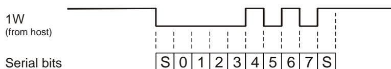
The QT1101 uses push-pull drive to transmit data out on the 1W line back to the host. When the stop bit level is established, 1W is floated; for this reason, a pull-up resistor should always be used on the 1W pin to prevent the signal from drifting to an undefined state. A 100K ohm pull-up resistor on 1W is recommended, unless the host uses open-drain drive to the QT1101 in which case a lower value may be required (see prior paragraph).
