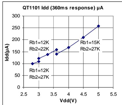
$C_x = 5\text{pF}$ ,  $C_s = 4.7\text{nF}$ ,  $T_a = 20^\circ\text{C}$ , No spread spectrum circuit (see Fig. 1.1).
